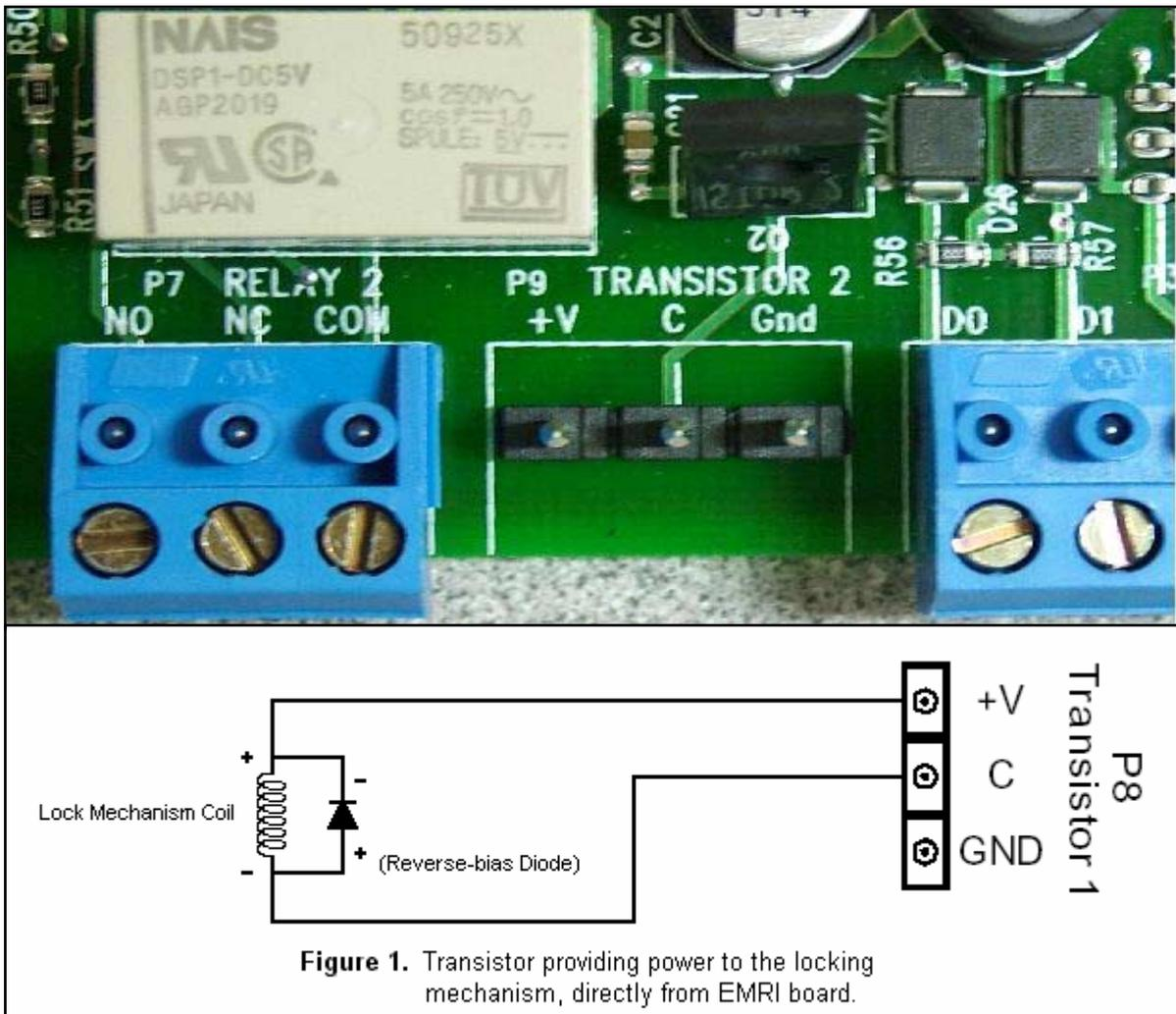
When the transistor output is not active, the collector "hovers" at a voltage close to +V. But when the transistor output switches to "active" the collector essentially "drops" to ground, creating a voltage potential between the collector (C) and (+V) pins, thus providing power to the locking mechanism.
