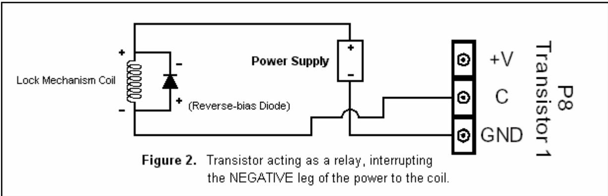
Please note that in **both** cases, a reverse-bias diode is employed across the coil, in order to prevent negative back-feed on the circuit. A diode of type **1N4001** is recommended.
