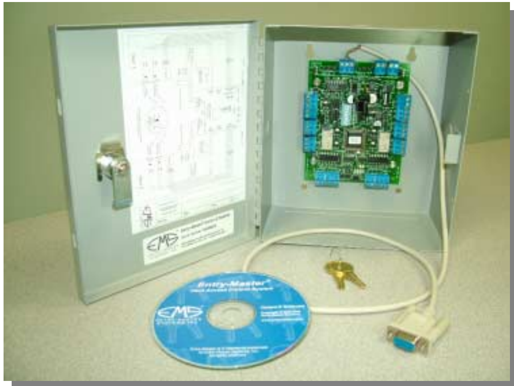
The Option-2 enclosure, circuit board, and communications cable
