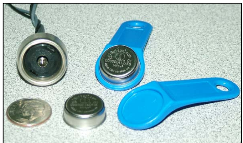
iButton readers, tokens and fobs shown next to a dime for comparison purposes.
